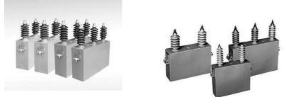
**Composition:** A capacitor is a passive two-terminal electrical component used to store energy in an electric field. The forms of capacitors vary widely, but all contain at least two electrical conductors separated by a dielectric (insulator). Most large capacitors consist of metal foils separated by a thin layer of insulating film. Prior to 1979, capacitors contained PCB oil as a dielectric fluid.
